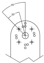
The gearbox mounting holes in the mounting bracket allow the motor and drive to be installed at 4 angles to suit different anchor well configerations. Another 8 adjustment angles are available at 30° and 45° from each of the basic 4 mounting holes.
