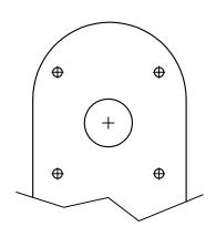
The gearbox mounting holes in the mounting bracket allow the motor and drive to be installed at 4 angles to suit different anchor well configerations. Another 8 minor angle ajustments are available between the gearbox and gearbox flange.
