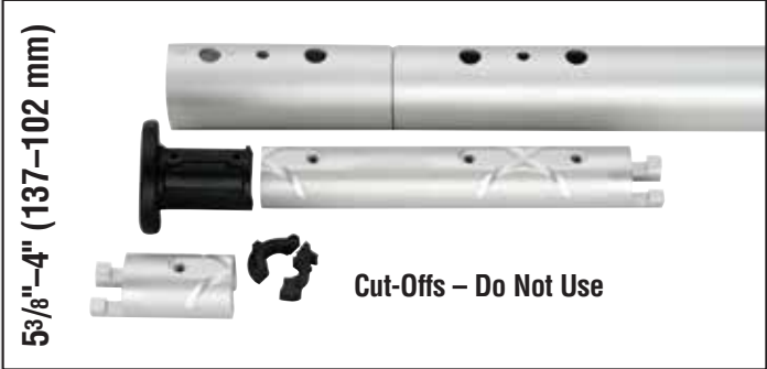
53/8"-4" (137-102 mm) Do not use plastic bushing above top connector. Cut connector right at cross formed by glue dispersion channels. Use single foil screw in top foil only.
