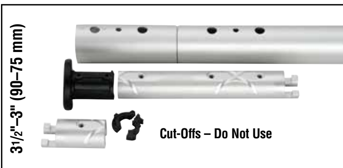
3 1/2"-3" (90-75 mm) Do not use plastic bushing above top connector. Cut connector right at cross formed by glue dispersion channels. Use single foil screw in top foil only.
