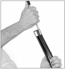
Snap foil into place by pulling aft with one hand, while sliding foil up with the other. Use heat gun.
