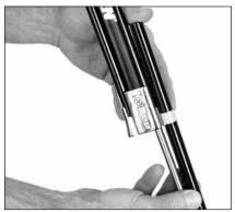
Measure length from feeder to bottom of exposed stay, for lower spacer tube length.
