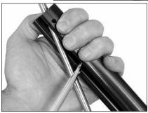
Splay foil with screwdriver and pull onto stay. Once foil is started, stop to install trim cap.
