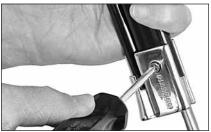
Coat screw with blue Loctite<sup>®</sup> and tighten. If screw does not thread, check alignment.
