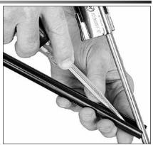
Cut, splay, and snap tube into place.
