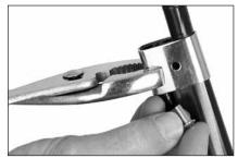
Place trim cap on foil so slot is aft, with large hole on starboard. Squeeze together with pliers. Put blue Loctite<sup>®</sup> in barrel nut. Install two-piece screw and barrel nut with Phillips screwdriver.
