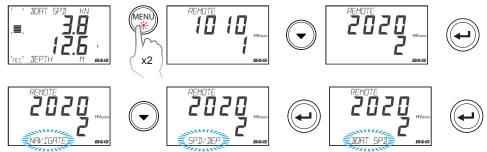
Use the up/down and **Enter** keys to navigate to a variable and select the variable to display. Exit with **Page** key.
