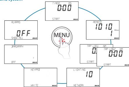
Press the **MENU** key to access the menu options i.e. the first menu option is TIMER, then REMOTE etc. - selecting the options clockwise as per the above illustration. Press **Page** to exit from menu system and return to last active page.
